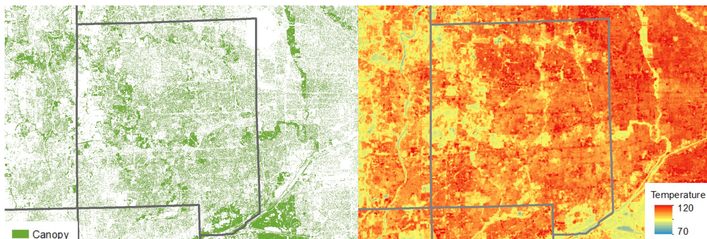
Figure 15: The image on the left shows tree canopy and on the right shows surface temperature. Surface temperature was calculated using a LandSat8 image from July 2017. Areas that have higher tree canopy tend to have lower temperatures.
