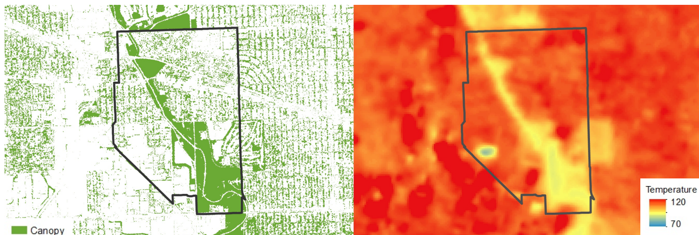
Figure 13: The image on the left shows tree canopy and on the right shows surface temperature. Surface temperature was calculated using a LandSat8 image from July 2017. Areas that have higher tree canopy tend to have lower temperatures.
