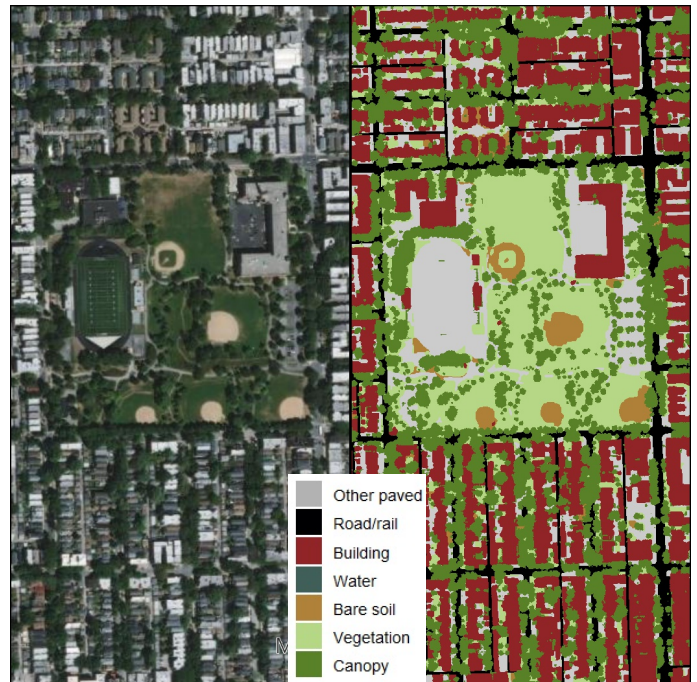
Figure 1: Comparison of imagery and land cover map. Seven types of gray and green infrastructure are in the land cover map.
